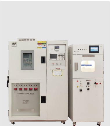
模拟EV车高频电晕老化试验仪器 Simulation EV vehicle high frequency corona aging test equipment
