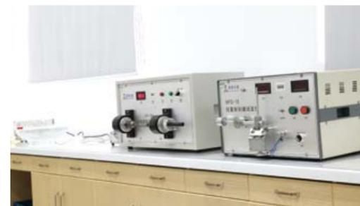
Scrape resistance tester 往复耐磨测试仪
