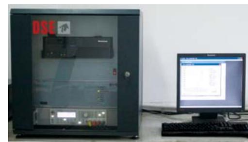
Dielectric loss tester 介质损耗测试仪
